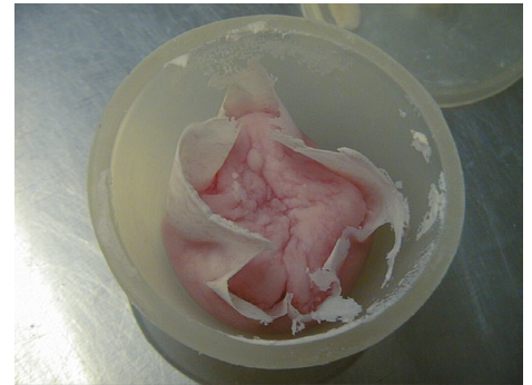
7.17 Acrylic ready to pack, pulls cleanly off bowl when squeezed.
