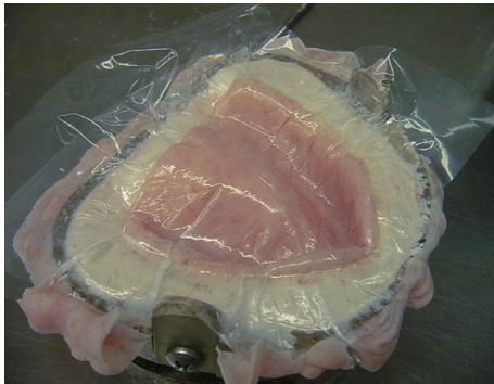
7.21 First press. Acrylic flash to be trimmed away, small amount of acrylic added where needed. Note wrinkles from cellophane.
