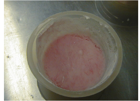
7.16 Acrylic not yet ready to pack, observe grainy and torn surface when silicone bowl is squeezed.
